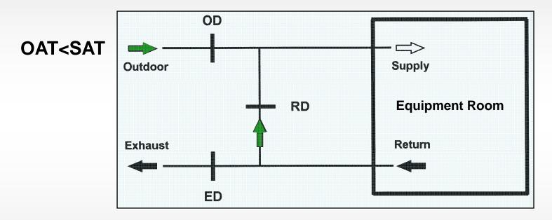
Air-side economizers are not only dependent on the return air temperature but also the supply air temperature and the outdoor conditions (climate).
